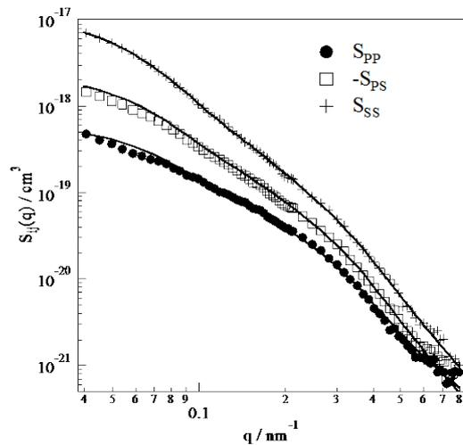
Fig.2 Partial scattering functions of rubber - filler systems
