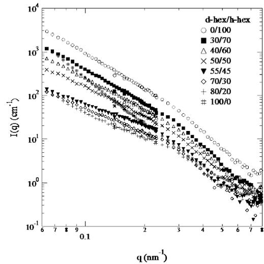
Fig.1 Scattering profiles for rubber-filler system swollen by d-hex/h-hex.
